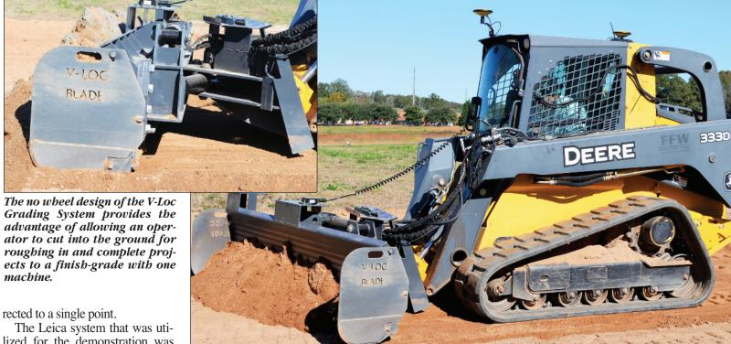
David's Dozer V-Loc Grading System — guided by GPS mastless technology — works flawlessly during a recent demonstration in Georgia.
